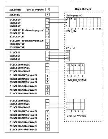
Figure 5–6 Bind Descriptor After Assigning Values
