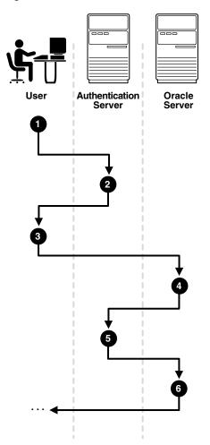
Figure 1–3 How a Network Authentication Service Authenticates a User
