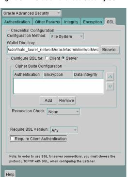
Figure 8–4 Oracle Advanced Security SSL Window (Server)
