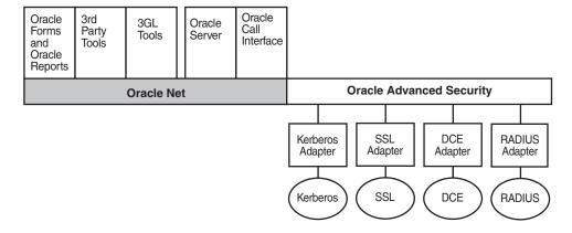
Figure 1–5 Oracle Net Services with Authentication Adapters
