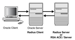
The Oracle database server acts as the RADIUS client, passing information between the Oracle client and the RADIUS server. Similarly, the RADIUS server passes information between the Oracle database server and the appropriate authentication servers. The authentication components are listed in Table 6–1:
