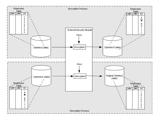
Figure 3-1 Transparent Data Encryption Overview
